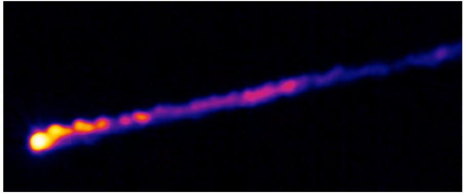
Thermal imagery of Space X Falcon 9 first stage performing supersonic retropropulsion in Mars relevant conditions in the Earth's atmosphere.
