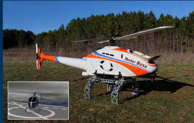
Landing on mountainous or pitching surfaces could be much safer with Rotor Buzz's flexible "legs" landing gear.
