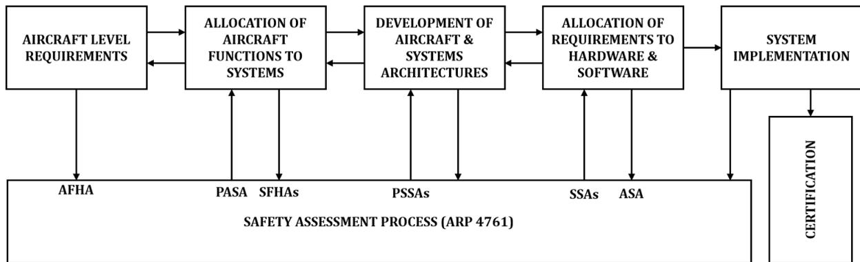
Figure 1: FSM approach for commercial transport aircraft.
